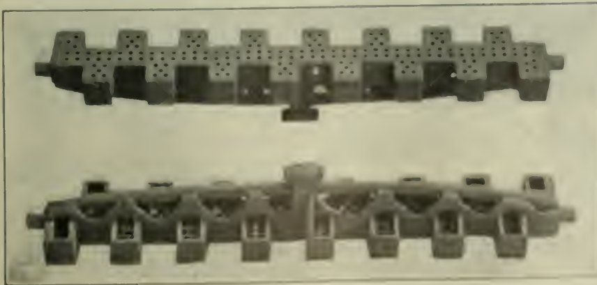
FIG. 5 TOP AND BOTTOM VIEWS OF A GRATE BAR
